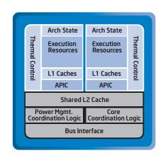
Intel® Core™2 Duo processor, based on Intel® Core™ microarchitecture, includes two complete execution cores, shared L2 cache, and intelligent power management features which deliver significantly greater performance-per-watt over previous-generation dual-core Intel® processors.
